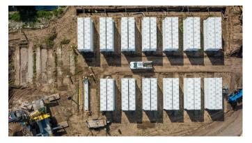
Goleta Energy Storage | Goleta, CA 60 MW BESS project 44 Tesla Megapacks BESS
